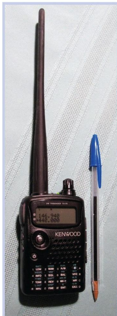
■ FIGURE 1. The Kenwood TH-F6A is a tri-band handheld FM transceiver for the 144, 222, and 440 MHz ham bands. Lots of buttons and menus make it a challenge to use.
